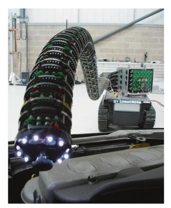
Fig. 8.9. 20-DOF snake-robot arm: 2.5 m reach, 90 mm diameter and payload capacity of 25 kg (image courtesy of OC Robotics)
