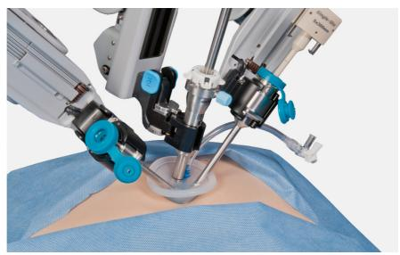
Fig. 1.8. The working end of a surgical robot, multiple tools working through a single small incision (image © 2015 Intuitive Surgical, Inc)
