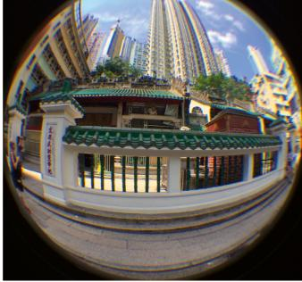
Fig. 11.17. Fisheye lens image. Note that straight lines in the world are no longer projected as straight lines. Note also that the field of view is mapped to a circular region on the image plane
