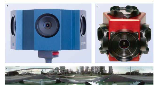
Fig. 11.27. Omnidirectional camera array. **a** Five perspective cameras provide a 360° panorama with a 72° vertical field of view (camera by Occam Vision Group). **b** Panoramic camera array uses six perspective cameras to provide 90% of a spherical field of view. **c** A seamless panoramic image ( $3760 \times 480$  pixels) as output by the camera **a** (photographs **a** and **c** by Edward Pepperell; image **b** courtesy of Point Grey Research)
