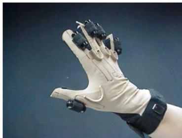
Figura 1.6: *Immersion's CyberGlove*
